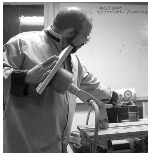
A vacuum pump can also be adapted as a stationary vise for carving or other applications. Carl mounted this articulated vacuum arm in a portable hobby vise.
