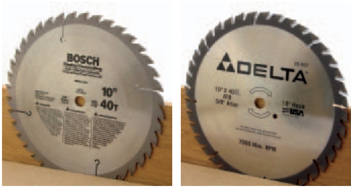
General purpose 10" blades often feature 40 teeth, an ATB grind, and a 15- to 20-degree hook angle.
