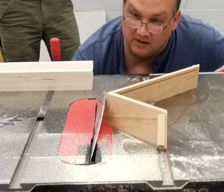
Steve sets the saw blade to match the corners
