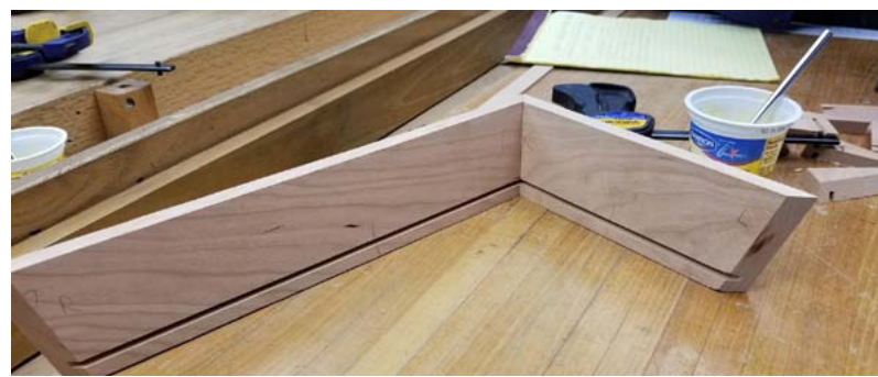
Two sides show grooves for beveled bottom
