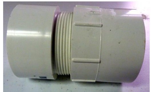
Schedule 40 pipe fittings are the raw material for the threaded insert
