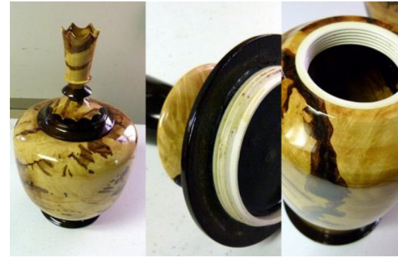
Composite view of the urn and finished male and female threaded components
