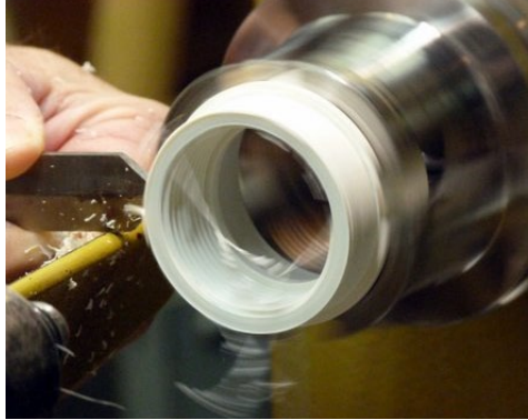
John cut down the outside diameter to fit into the urn
