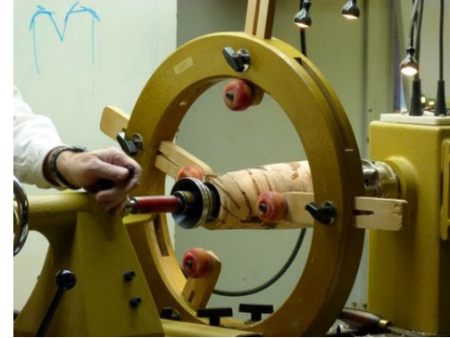
The insert unit is glued into the urn with help from two chucks and a bowl steady rest
