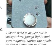
in the magnet cup to allow removal of the magnet if necessary
