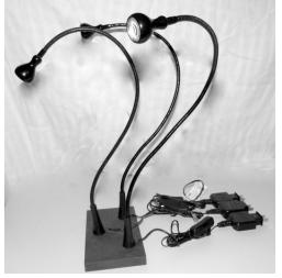
Finished workstation liaht can be moved anywhere on the lathe -- stays secure with the magnet mounts
