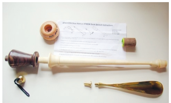
Components of a shoe horn project. All the brass pieces come in the kit.
