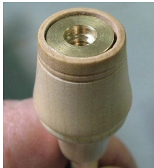
Recess the coupler end to have the couple sit flush
