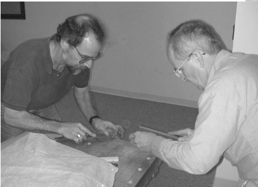
Steve Mapes and Tom Osborne use files and tempered spring steel to make their own tools to create beading and string inlay.
