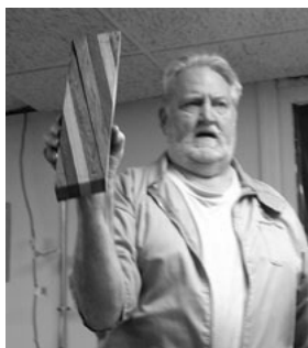
Pieces are then flipped and re-glued to form parallelogram
