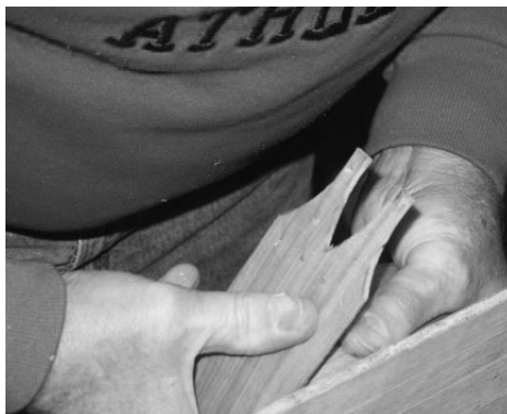
Bending a cherry band around the form. Swallow-tail joint visible.
