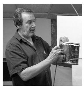
A coffee can makes an excellent receptacle for excess paint spray. A tee shirt scrap provides a filter.
