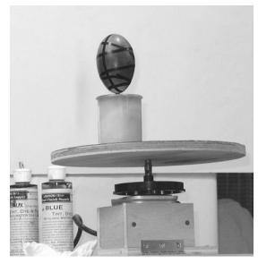
A turntable with a slow motor can be used for airbrushing -- here an egg is masked and colored
