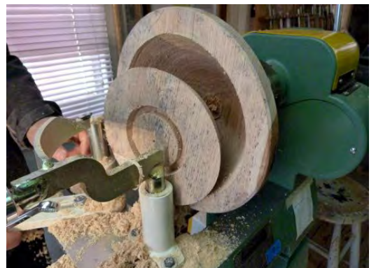
The cored bowl blank pops out of the original timber: two oak bowls!
