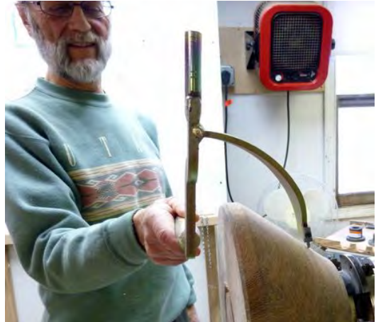
The process begins by 'eyeballing' the intended radius, leaving enough material to form a tenon for the cored blank
