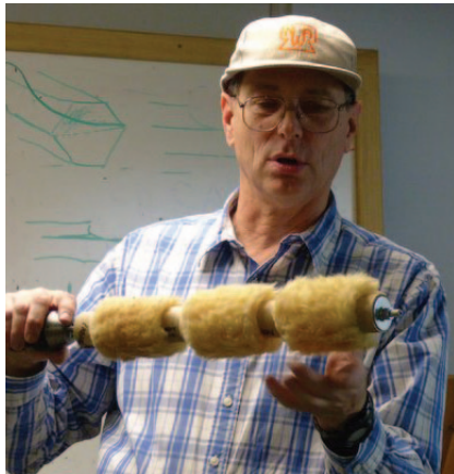
John Franklin showing a buffing system constructed of paint rollers by Steve Sherman
