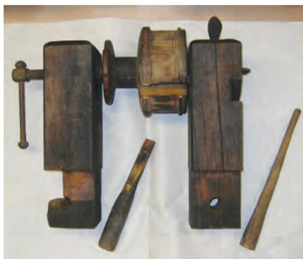
Hurley lathe headstock and pulley assembly
