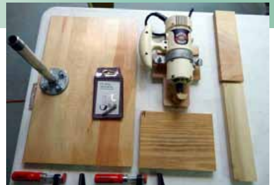
Fluting jig components: platform, sled, and stop blocks
