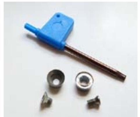
HSS cutter on left, carbide version on right. Note the carbide requires a longer screw. Both need Torx key.
