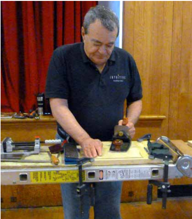
Joe Kennedy uses a scraper plane
