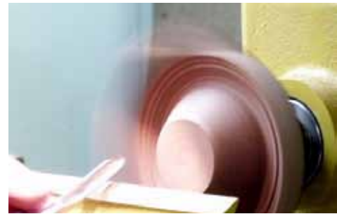
The bottom is turned, shaping the wings and bottom of the bowl
