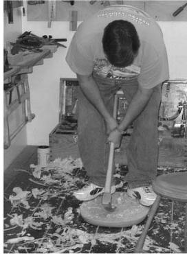
*Using an adz to hollow the seat*
