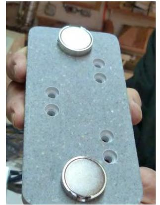
*Plastic base is drilled out to accept three Jansjo lights and two magnets. Notice the notch in the magnet cup to allow removal of the magnet if necessary*
