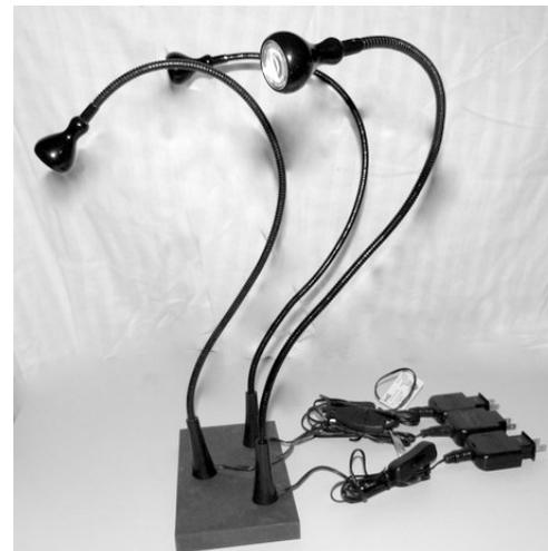
*Finished workstation light can be moved anywhere on the lathe -- stays secure with the magnet mounts*
