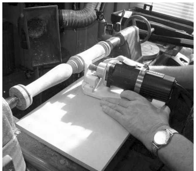
The flute is cut by sliding the jig along the table
