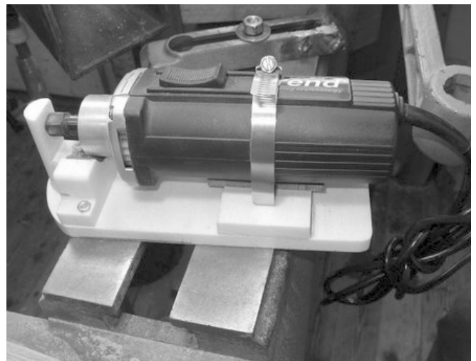
T3 in Steve's jig - nose piece is rounded
